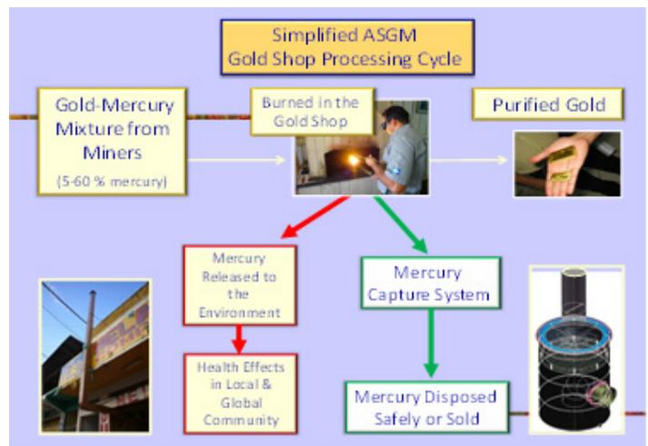
A simplified schematic of amalgam burning and mercury release in a gold shop. The MCS can help reduce the risk of exposure to mercury for gold shop owners, adjacent community members, and the global environment. Photos courtesy of the U.S. EPA.
