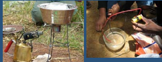
Miner re-activating mercury using a radio battery; the process takes about 10 - 20 minutes
