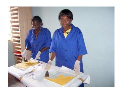
A razor blade shall be used to scrape dried sample in the sample container
