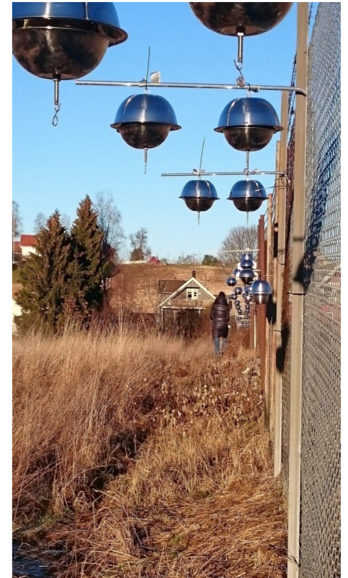
Figure 1: Phase 1 PUF-PAS deployment in Kjeller, Norway (Bohlin Nizetto et al., SETAC 2018 Rome)
