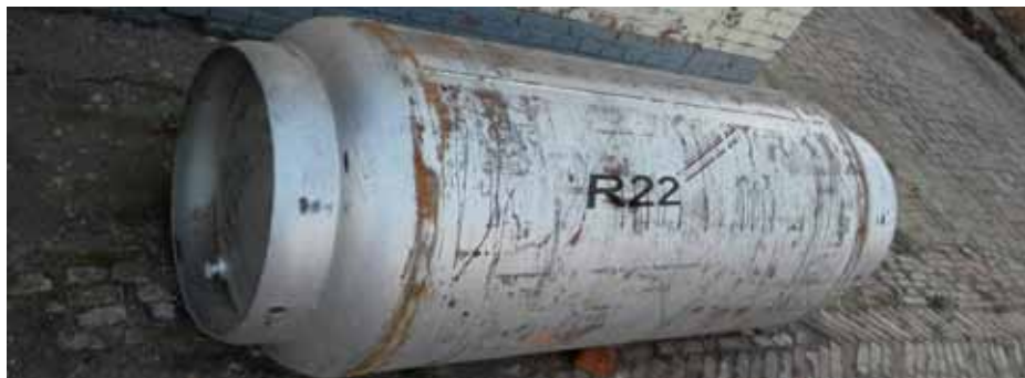
Figure 24. Cylinder surface marked with R22
