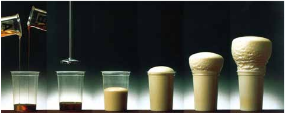
Figure 3. Blowing procedure of PU foam
