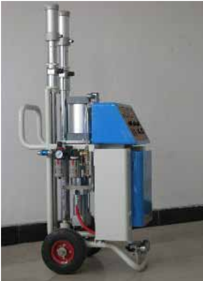
Figure 4. PU foam-spraying machine
