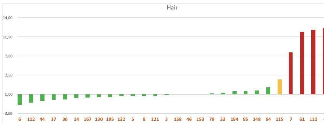
Figure 7 Results delivered for human scalp hair test sample expressed in z-scores for individual laboratories shown via laboratory codes.
