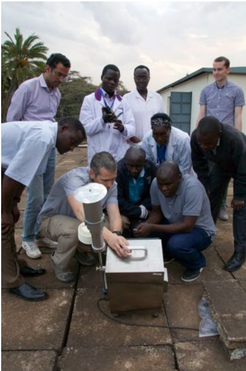
Operating active sampler - Kenya (photo by RECETOX)
