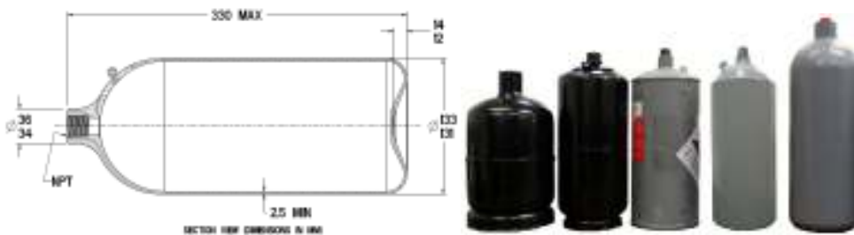
Figure 3.2 - Design of 3L flask - 76 lb or 34.5 kg ( SOURCE: Oak Ridge Laboratory, 2009)
