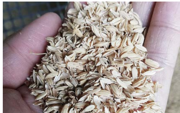
Fig. 15 Rice husk used to adjust moisture content at a composting plant in Nagai City, Japan
