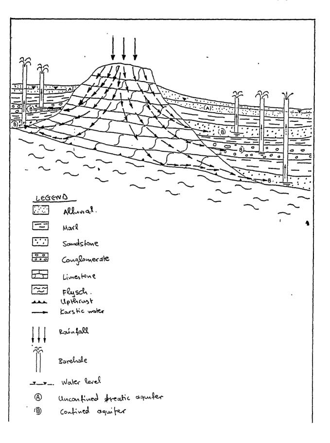
i (A) ì a  $\sim$  $\sim$ • C (<u>B</u>) O Q à (B) ŧ LEGEND Alluvial deposits day Conglomerate Marl water level χ. Borchole Unconfined freshic aquifer ٩, (B) Confined aquifer
