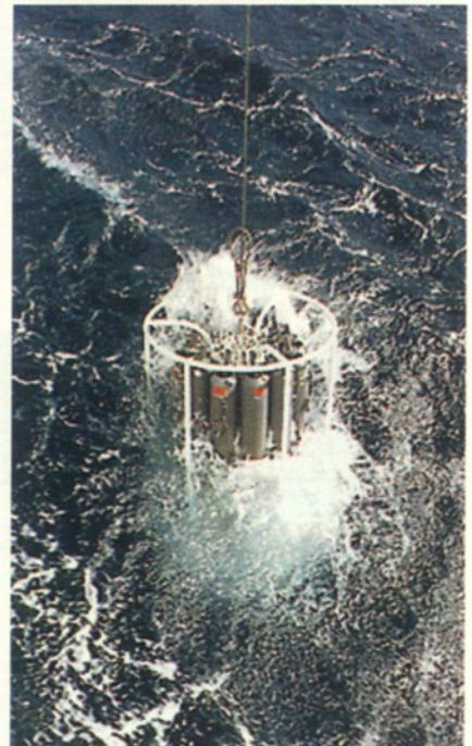
Mission in Mediterranean March 1998: Launching the sampling rosette (Photo: N. Bensoussan Marseille Oceanology Centre)
