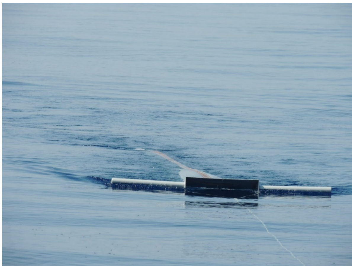
Figure 3: Manta net being operated in calm sea, outside of the bow wave caused by the spinning of the propeller (Photo: © Christos Ioakeimidis, UNEP/MAP).
