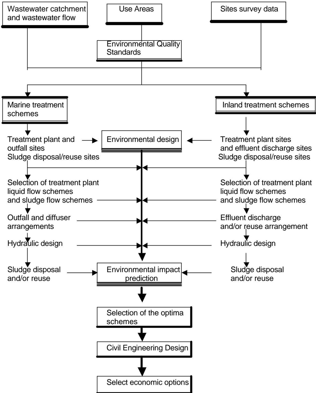
**Figure 4. Wastewater sanitation schemes - design flowchart**
