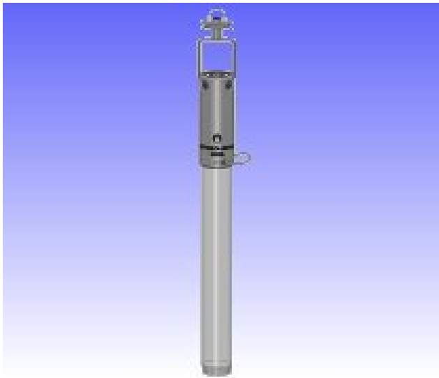
Figure 2: Gravity corer (picture from Hydro-Bios, Germany).
