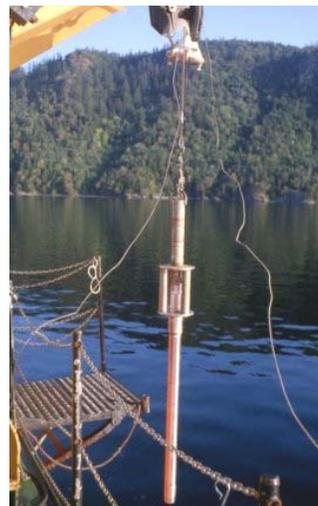
Gravity core sampler
