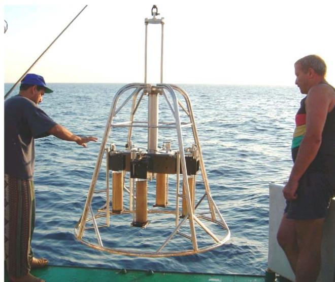
Figure 3: Multi-core sampler.
