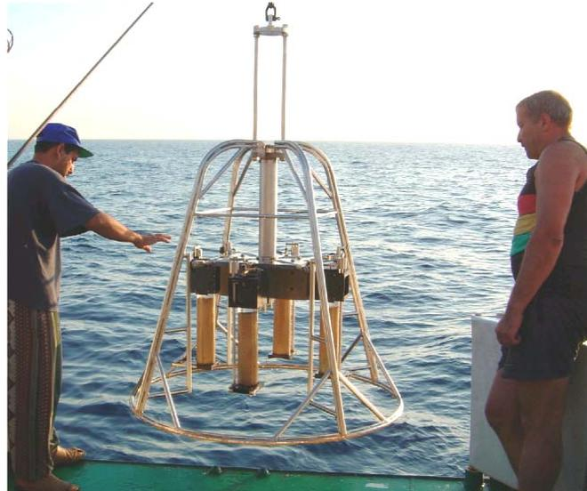
Figure 3: Carottier multitubes.
