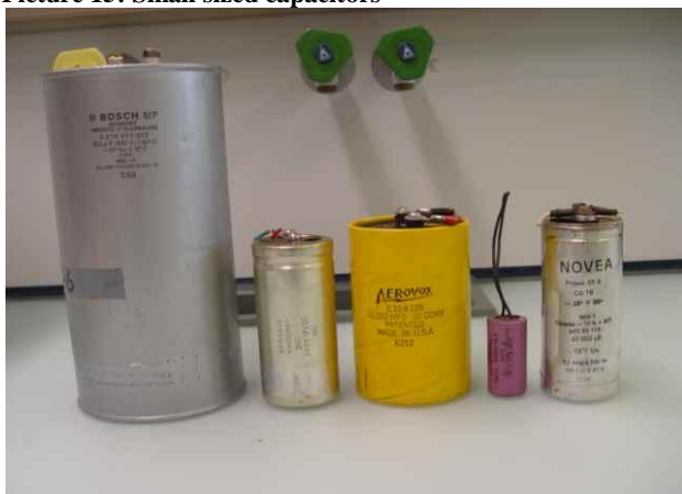
Picture 15: Small sized capacitors
