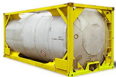
Picture 66: 20' tank container liquids
