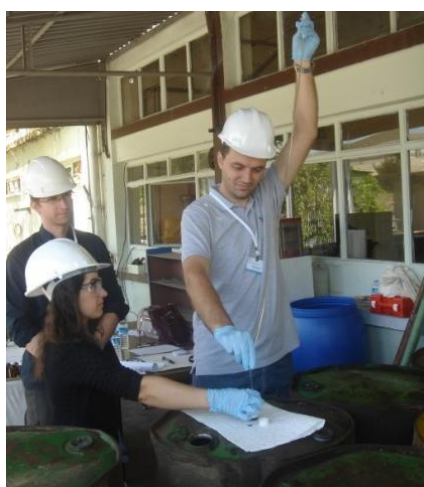
Picture 11: Sampling of oil drums
