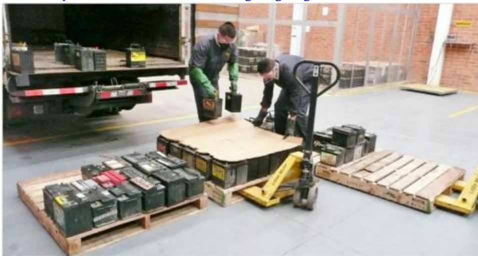
Fig. 12: Packaging of used lead batteries ready to transport – good example
