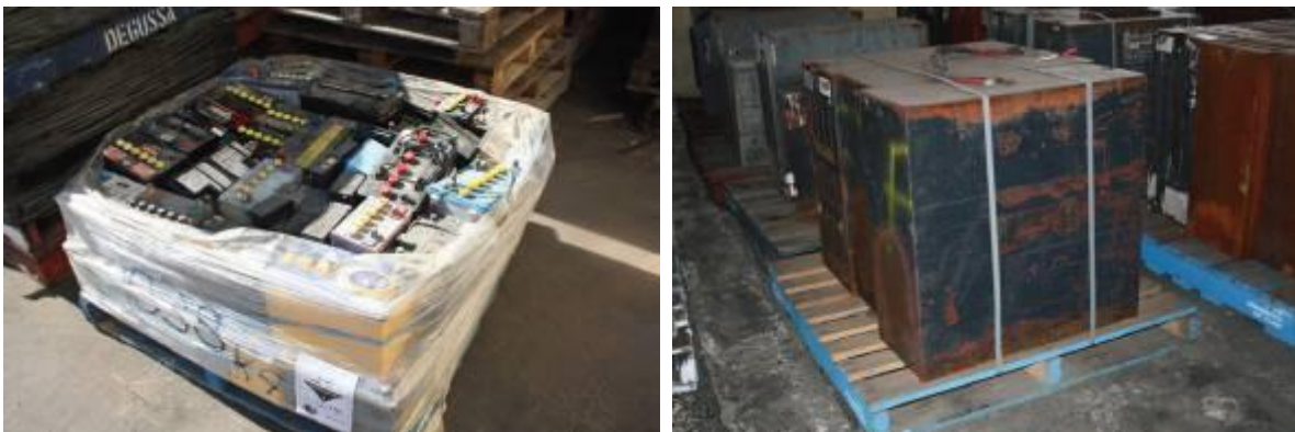
Fig. 40: Examples of bad packaging before transport, ABRI [26].
