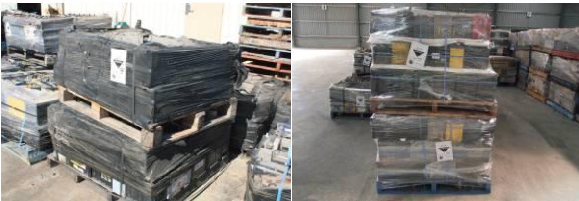
Fig. 39: Examples of bad packaging before transport, ABRI [26].
