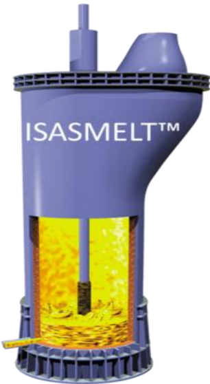
Fig. 26: Example of ISA Smelt furnace [31]
