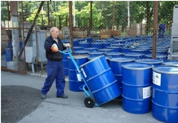
Picture 82: Safety Drum lift
