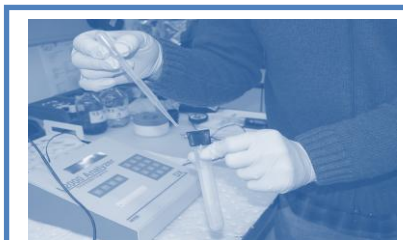
Screen the oil sample by Clor-N-Oil or L2000 DX
