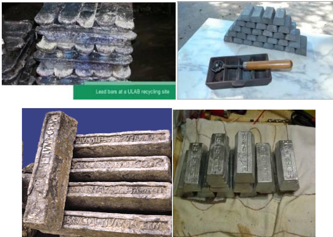
Fig. 32: Lead bars as the final product
