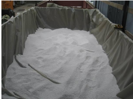
Picture 70: Covering the bottom with absorbent material
