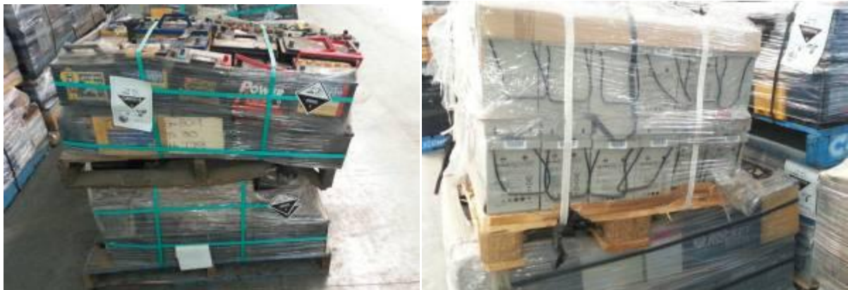
Fig. 41: Examples of bad packaging before transport, ABRI [26].
