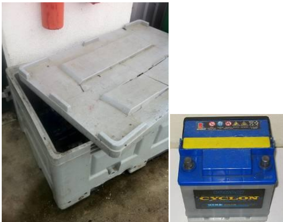
Fig. 7: Container for separate collection of used lead batteries in vehicle service
