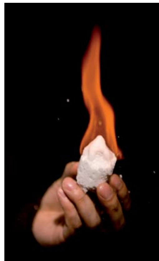
The icy material of methane hydrates looks like ice, but burns if ignited. Source: National Research Council Canada
