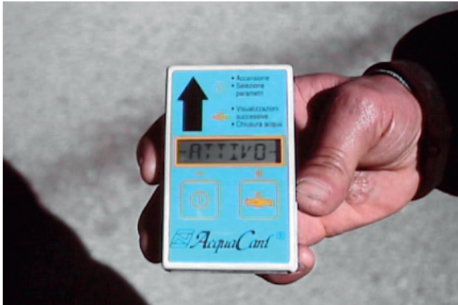
Electronic card, the portable device enabling farmers to decide on when and how much water they want to apply, monitor their water consumption and check on the remaining volume of water Credit: Dr. Nicola Lamaddalena
