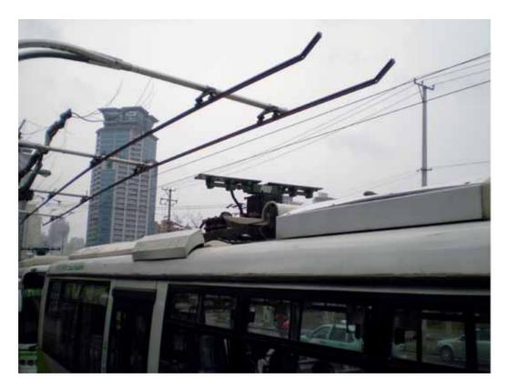
The conductor of the supercapacitor trolleybus rises to the overhead charger in the terminal station on Line 11.
