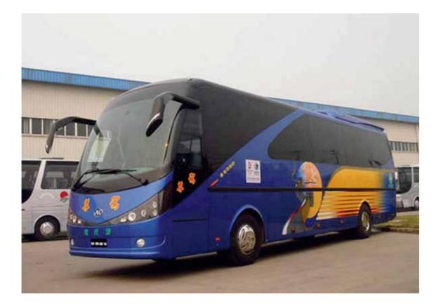
A prototype battery-supercapacitor all-electric bus
