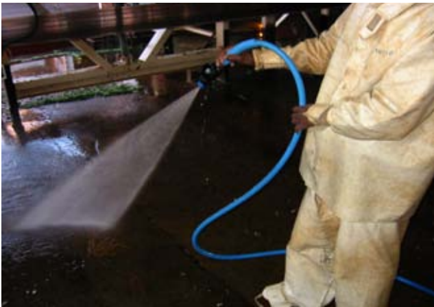
Figure 27: Using an open hose for floor cleaning 29
