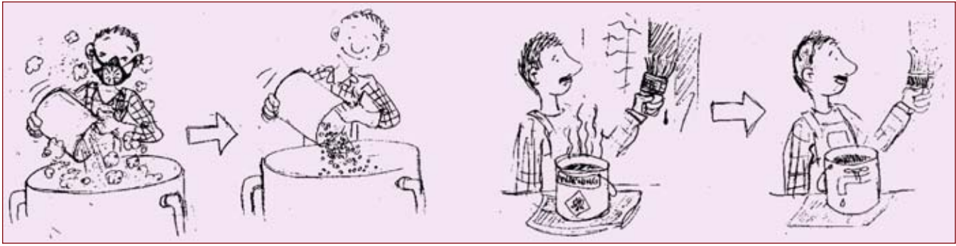
Figure 46: Using pellets instead of powders and using water-based paint instead of oil-based 96
