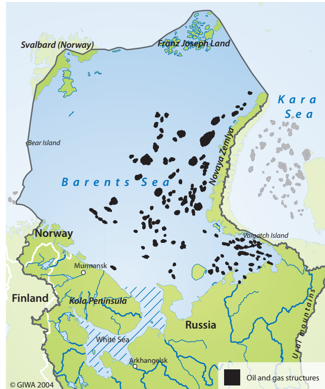
Figure 12 Oil and gas structures of the Barents and Kara Seas. (Source: Denisov 2002)
