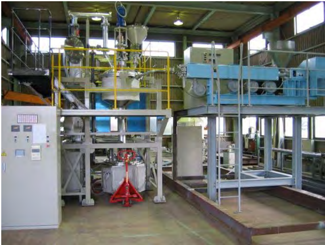
Figure 8.5: Fuel Oil Production Plant YUKAKI MYF125
