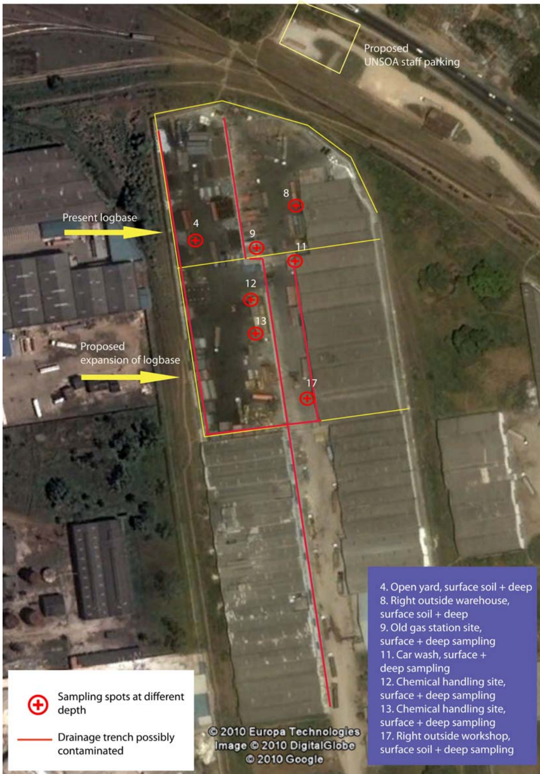
Figure 2. Sampling spots where samples were taken at two or three different depths.
