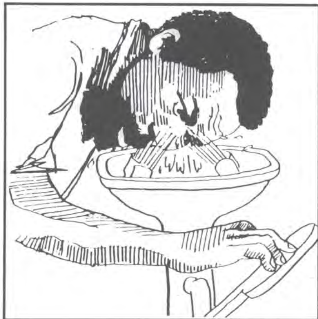
Figure 56. Emergency showers and eye-wash points should be provided in close proximity to workstations where hazardous chemicals are used
