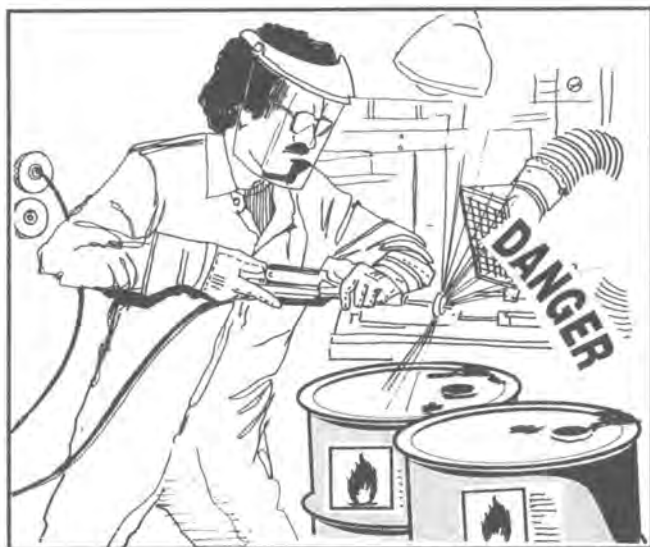
Figure 19. The open flame from welding and cutting torches can cause the ignition of flammable vapours
