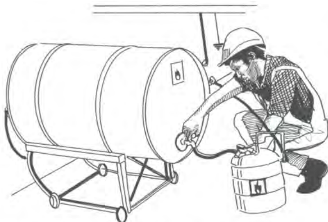
Figure 37. A specially designed container for the transfer of small quantities of flammable liquids
