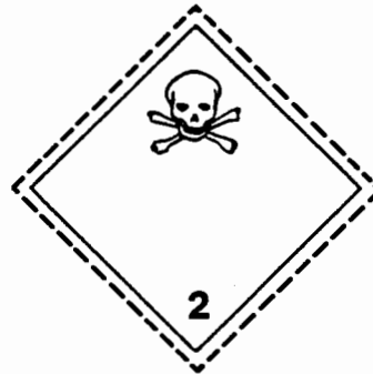
Poison (toxic) gases Symbol (skull and crossbones): black Background: white
