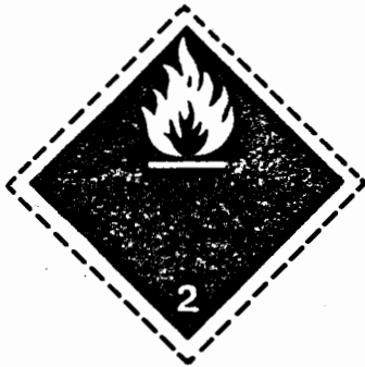
Inflammable gases Symbol (flame): black or white Background: red
