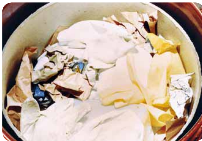
Compactable low level waste may include radioactive clothing, glass and building materials. Credit: Sellafield Ltd.
