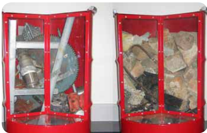
Interim packaging and storage of radioactive waste. Source: Nuclear Decommissioning Authority, United Kingdom
