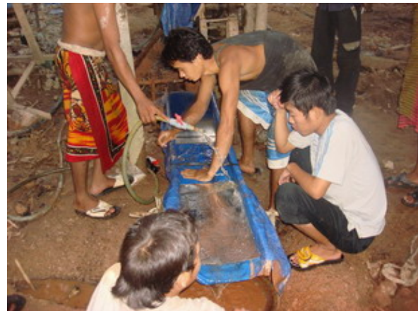
Miner washes the dirt out to obtain gold with mercury-amalgam
