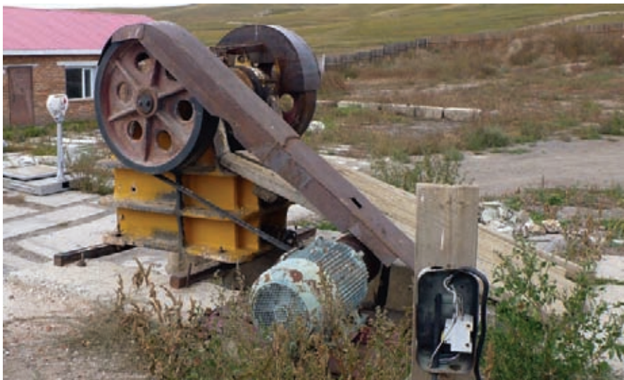
② Rocks are crushed down to 1-2 cm size using a jaw crusher
