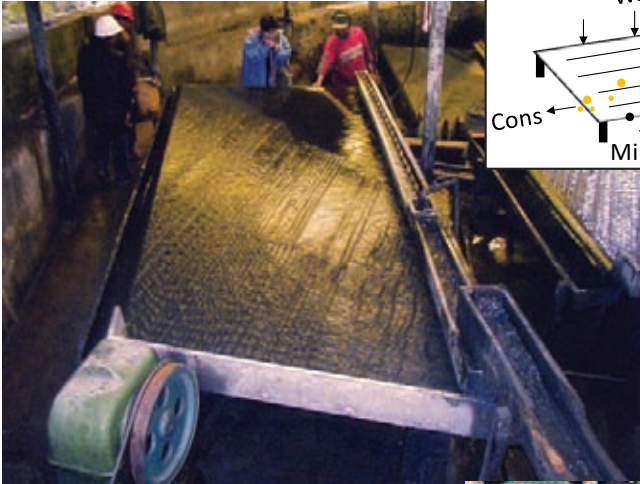
A large shaking table is used at a small-scale mercury free processing plant in Mongolia.
