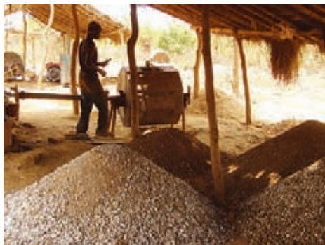
Rocks are crushed manually using hammers (not shown), and then milled using ball mills (Tanzania, 2010).
