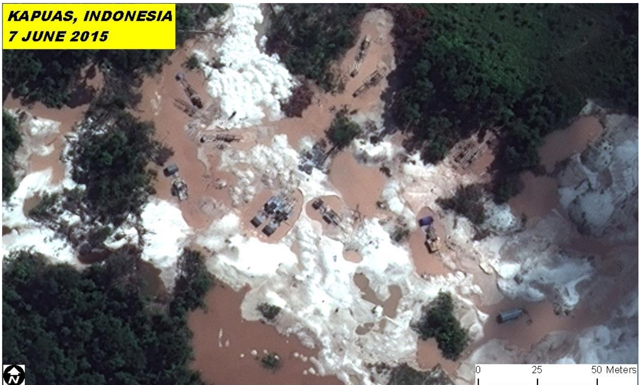
Figure 5: Kapuas (7 June 2015) – Mining activity in the form of dredges along the main river in Kapuas. A total of 13 dredges are visible in this image, many of which are composed of a square hut for four or five people at the end of a raft with a pumping unit and a long sluice.
