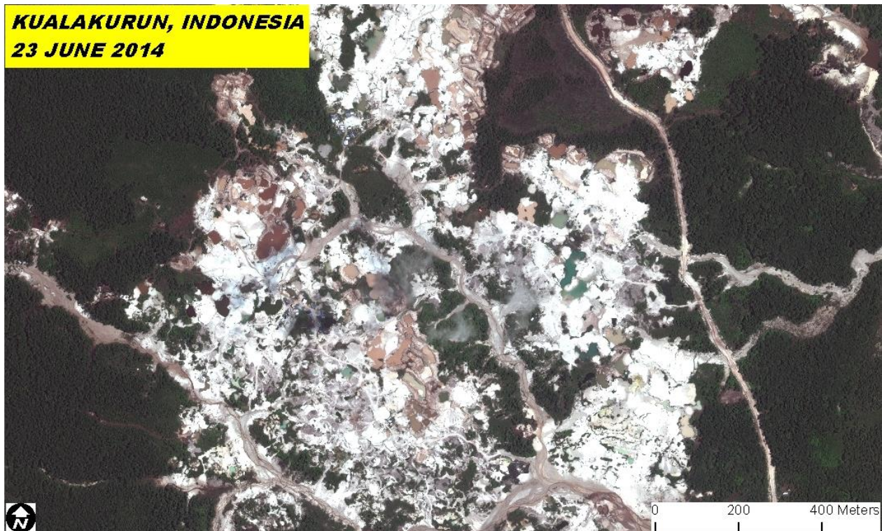
Figure 1: Kualakurun (23 June 2014) – Overview of open mine pits in northern and central Kualakurun. A few mining camps are visible, though for its large size there is limited observable mining equipment apart from two dredges and twelve possible sluices.
