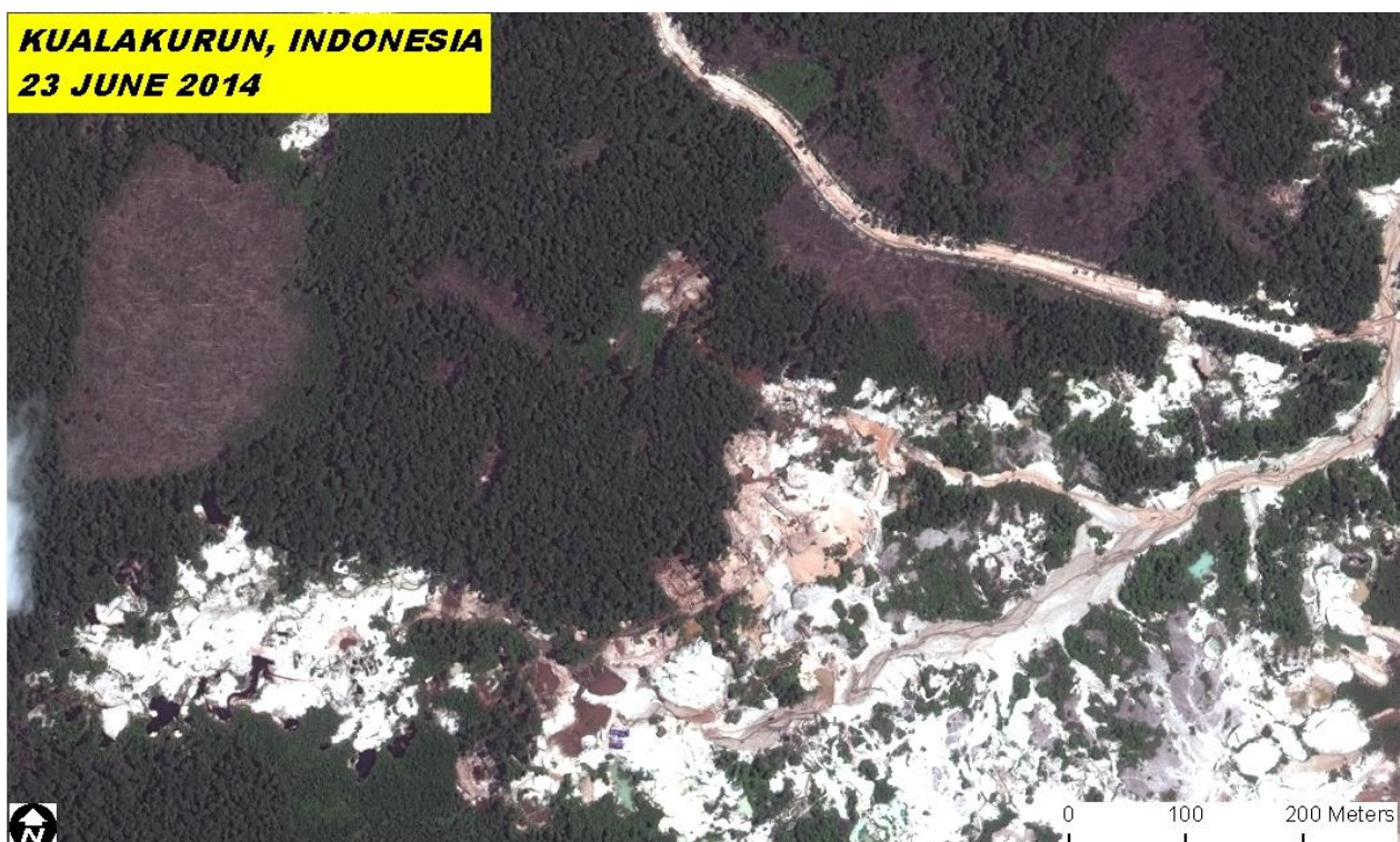
Figure 2: Kualakurun (23 June 2014) – Deforested areas and nearby mine pits in the northwestern part of Kualakurun. Some structures and possible sluices are also visible. Deforestation may be a precursor to open pit mining.
