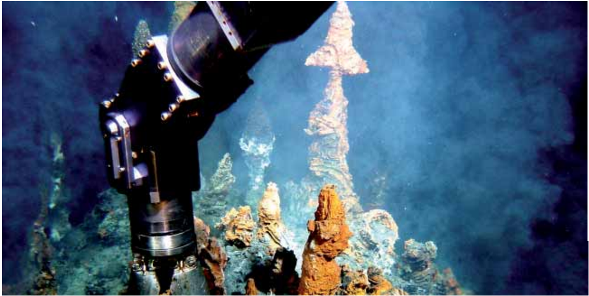
Sampling of hydrothermal vent chimneys in the North East Pacific at 260 metre depth using ROV Victor.
