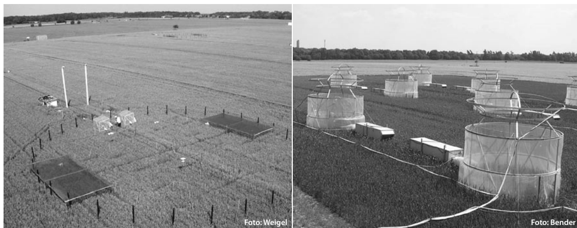
FIGURE 1. Field experiments on atmospheric climate change effects in agroecosystems at the Federal Agricultural Research Centre in Braunschweig (Germany) considering soil biodiversity. Left: One plot of the FACE (Free Air Carbondioxide Enrichment) experiment. Right: Open-top chambers to study effects of elevated ozone (O 3 ) concentrations.
