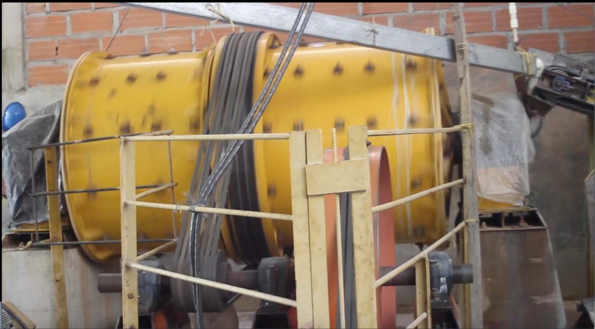
A large ball mill, with crushers feeding it the optimal sized material, liberates the gold without mercury.
