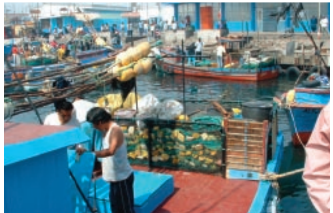
Fig. A6.8. Stored mainline in stern of fishing vessel. Note the main line with integrated floats and the wood planks holding hooks to the right.
