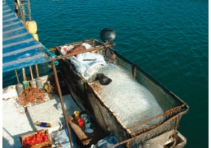
Fig. A2.9 An artisanal longline vessel in Arica using a monofilament mainline.
