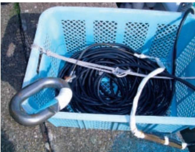
Fig. A5.10. The ring and electrical cord of the “shocker” device used by engan fishermen based in Kii-Katsuura to immobilize sharks. (Photos courtesy of T. Miyamoto.)
