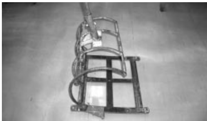
Fig. A5.8. Clamping device designed and used by one kinkai fisherman based in Kesennuma for immobilizing sharks. (Photo courtesy of T. Miyamoto.)
