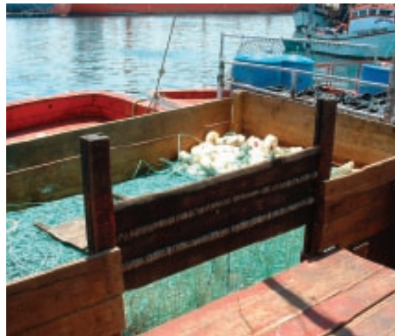
Fig A2.11. Multifilament mainline and hooks in stern of artisanal longline vessel.
