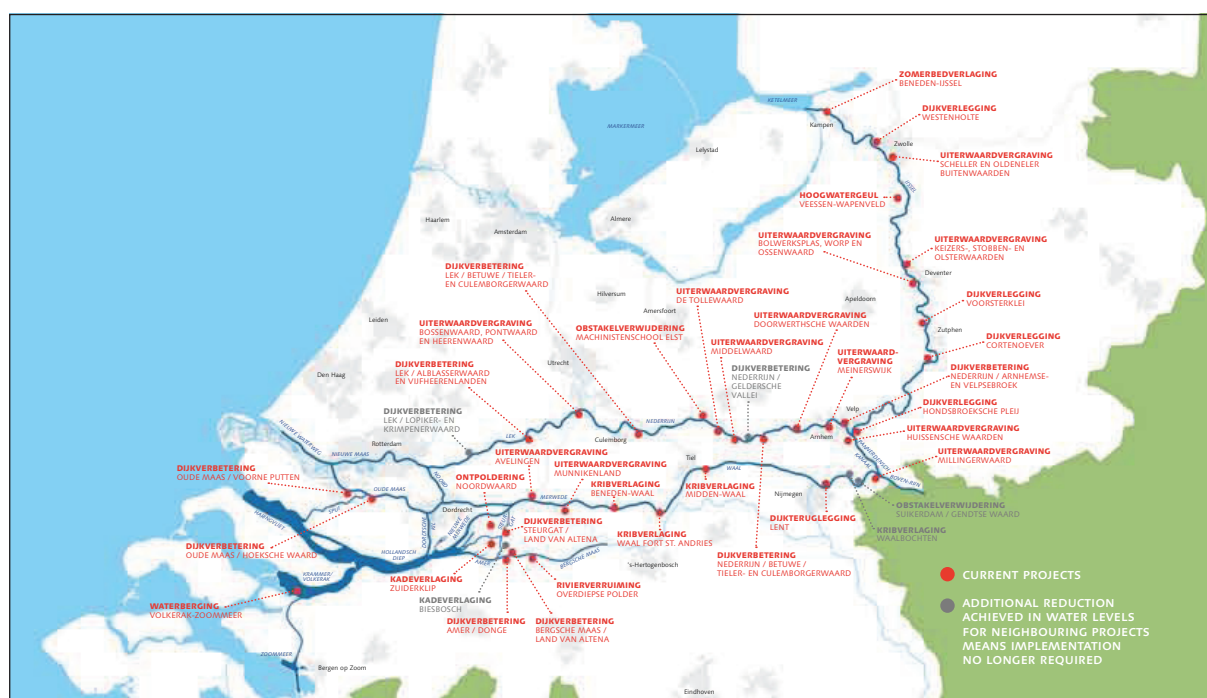
Figure 4. Intervention map of Room for the River Programme with the corresponding measures. Measures in 4 out of the 39 selected areas have been deemed unnecessary after reduction of water levels have been achieved in nearby areas. Adapted from Dutch Ministry of Water Management, Transport and Public Works, 2012
