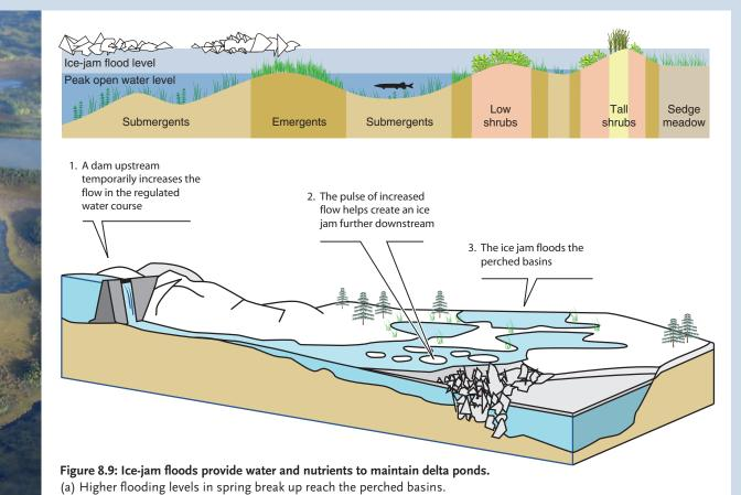
(b) An adaptation strategy: water released from the reservoir on the left increases the probability of ice jams and flooding of the ponds.
