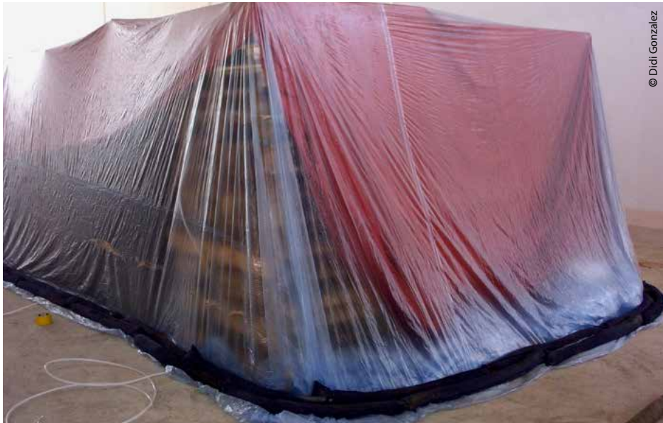
Stack of wooden pallets under MB fumigation to comply with ISPM 15 in the Philippines.
