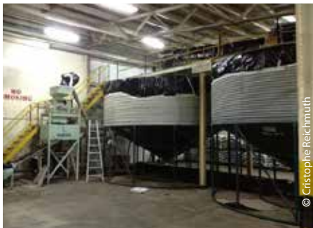
Silo fumigation with phosphine.
