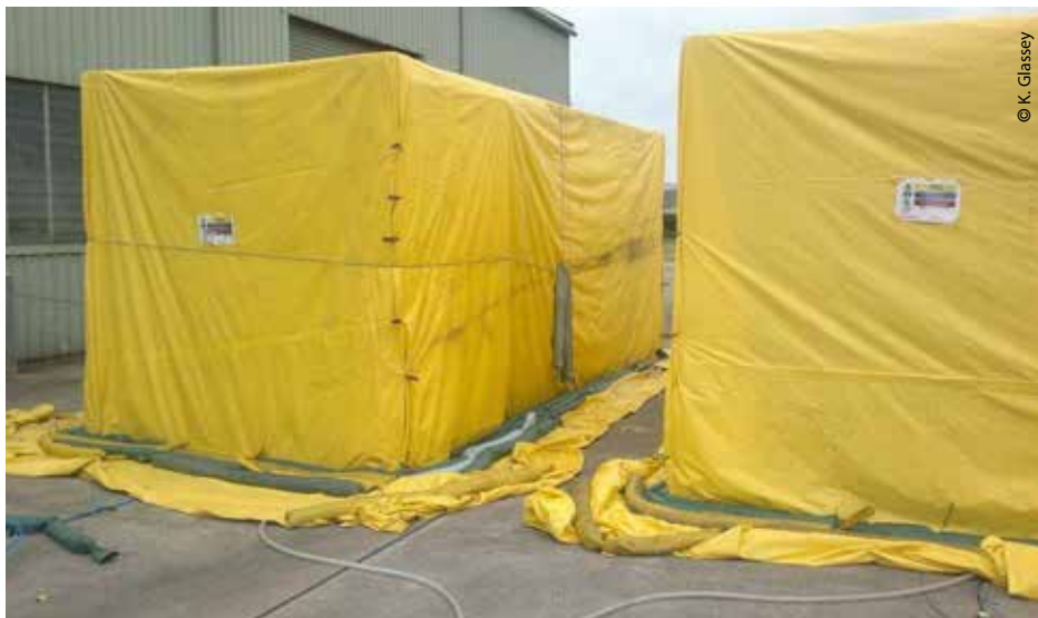
Good covers are essential to minimise MB leakage and ensure efficient MB use.
