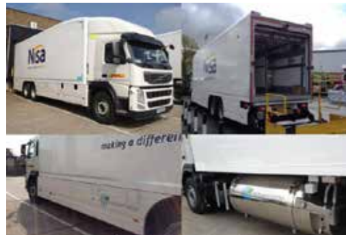
Fig. 2 natureFridge refrigeration system installed in track
