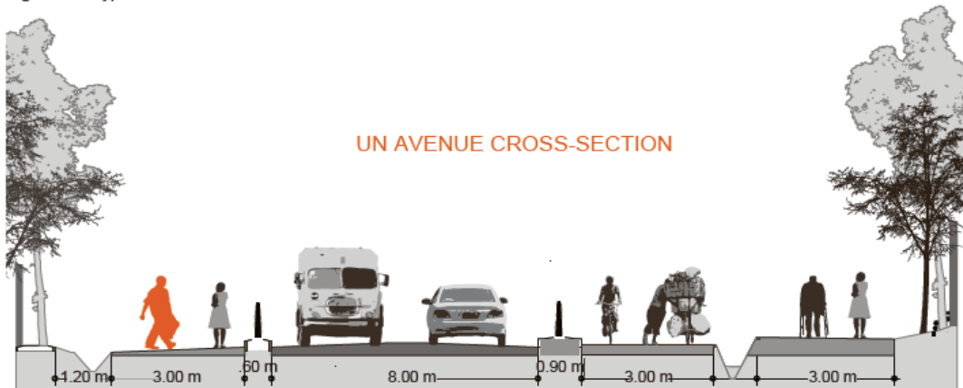
Figure 21: Typical Road Section of UN Avenue
