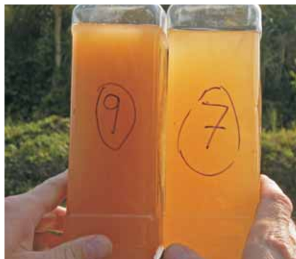
Water samples revealing high content of suspended sediments
