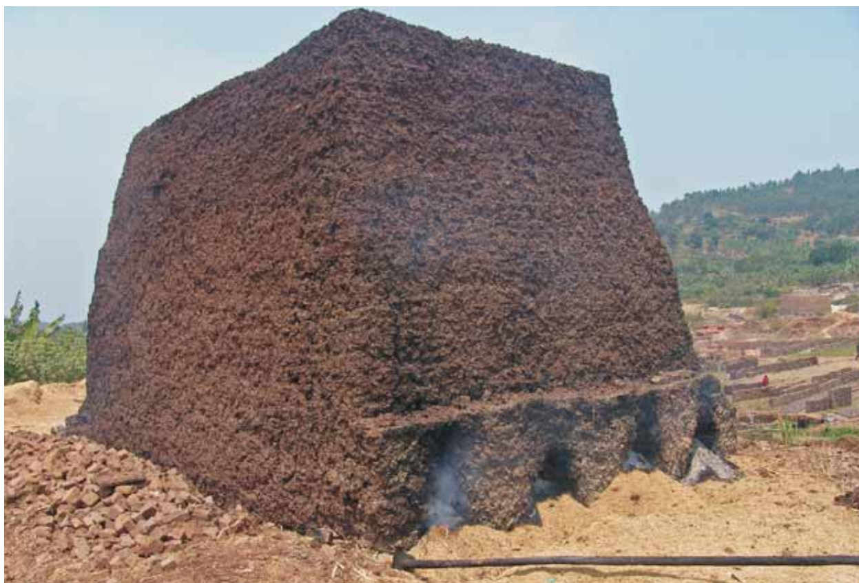
Following the ban on the use of firewood in brick kilns, fuel options remain crude, ranging from sawdust (above) to more polluting sources such as heavy fuels. While alternative technologies are more expensive, there are opportunities for improving the efficiency of traditional brick making
