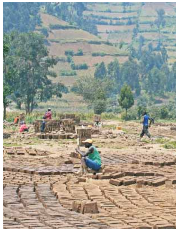
Residents in Nyabihu District produced sun-dried adobe bricks to reconstruct their homes destroyed by flood
