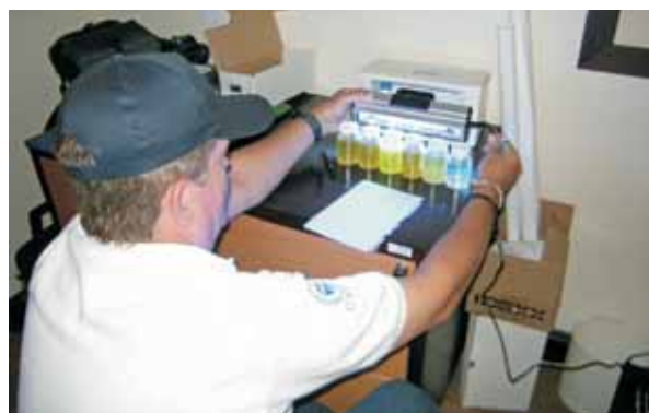
UNEP expert testing for the presence of coliforms in drinking water samples
