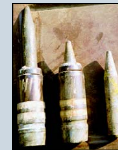
30mm DU munition: jacket and penetrator
