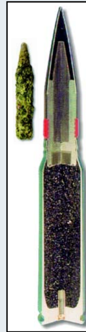
Corroded penetrator (left) and 30 mm DU munition profile
