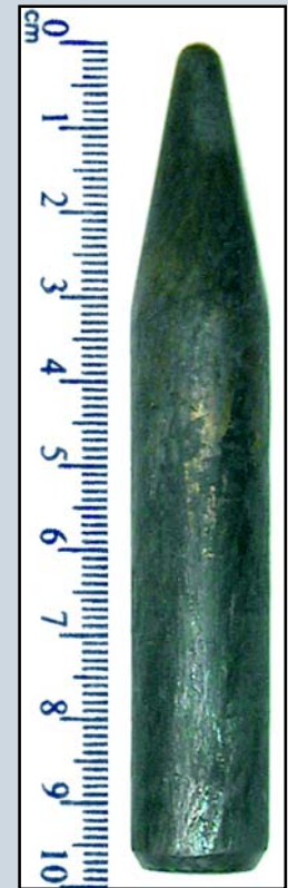
DU Penetrator in its original size
