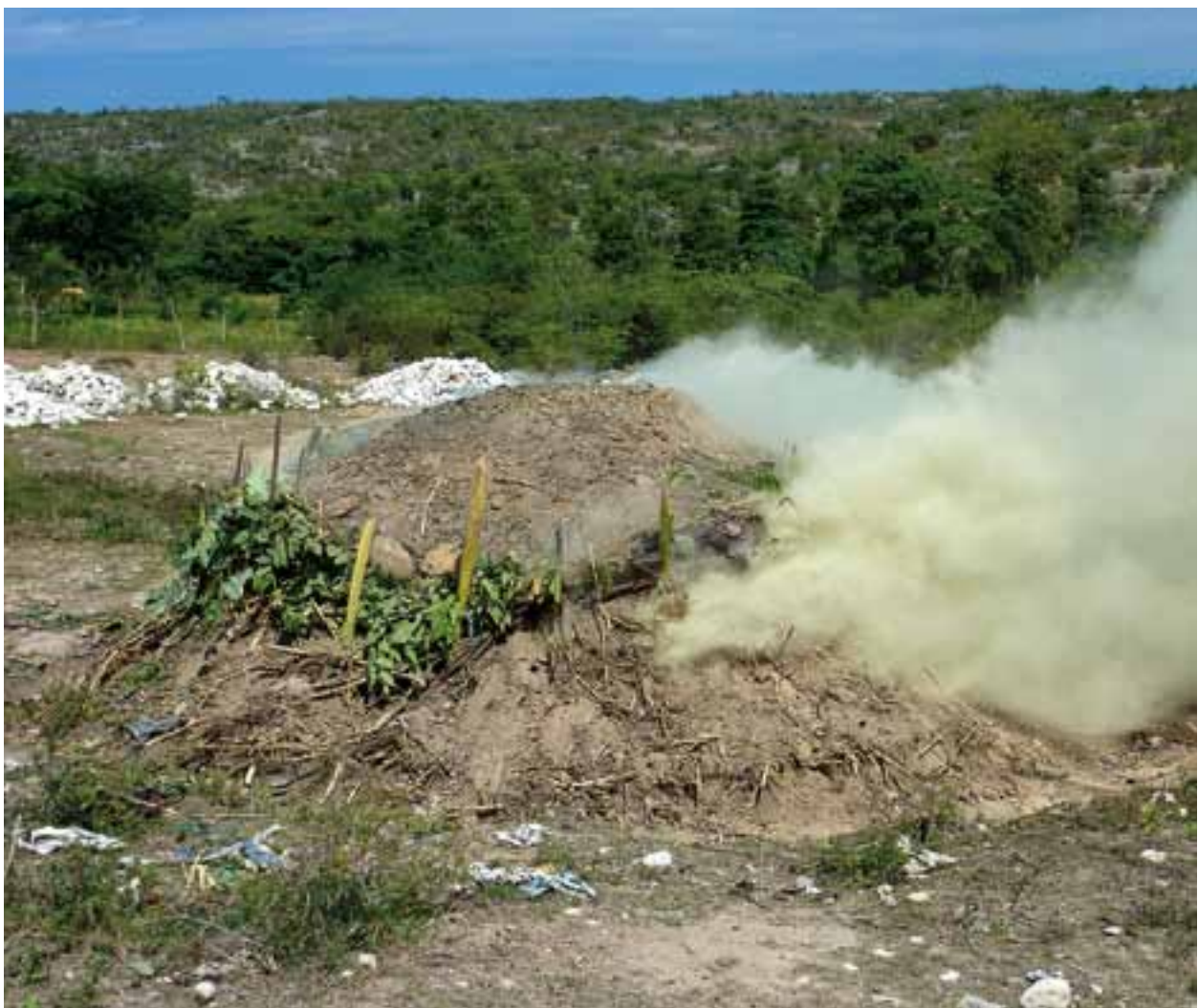
Charcoal is produced in charcoal kilns – such as this one in the lower part of the Pedernales Watershed – that turn wood into charcoal by drying it.
