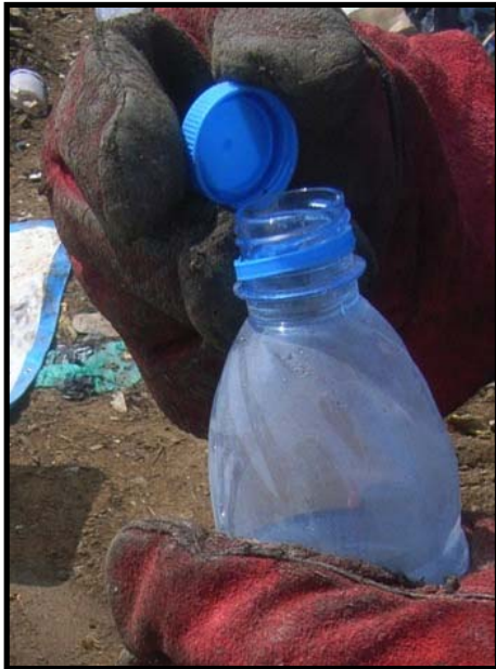
The HDPE cap from a PET water bottle being separated
