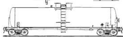
Low Pressure Tank Car Liquids (Closed Dome and Outlets on top) (131)
