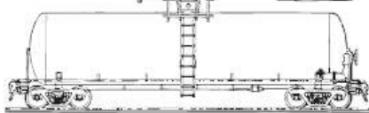
Pressure Tank Car Compressed Liquefied Gases (Closed Dome Only on top) (117)
