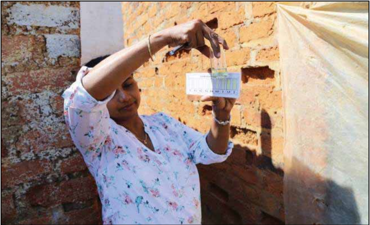
Simple visual colour comparators can be used for measuring residual chlorine and pH
