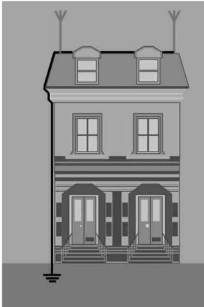
Figure 4.8 Air Terminal, down conductors and Earth termination
