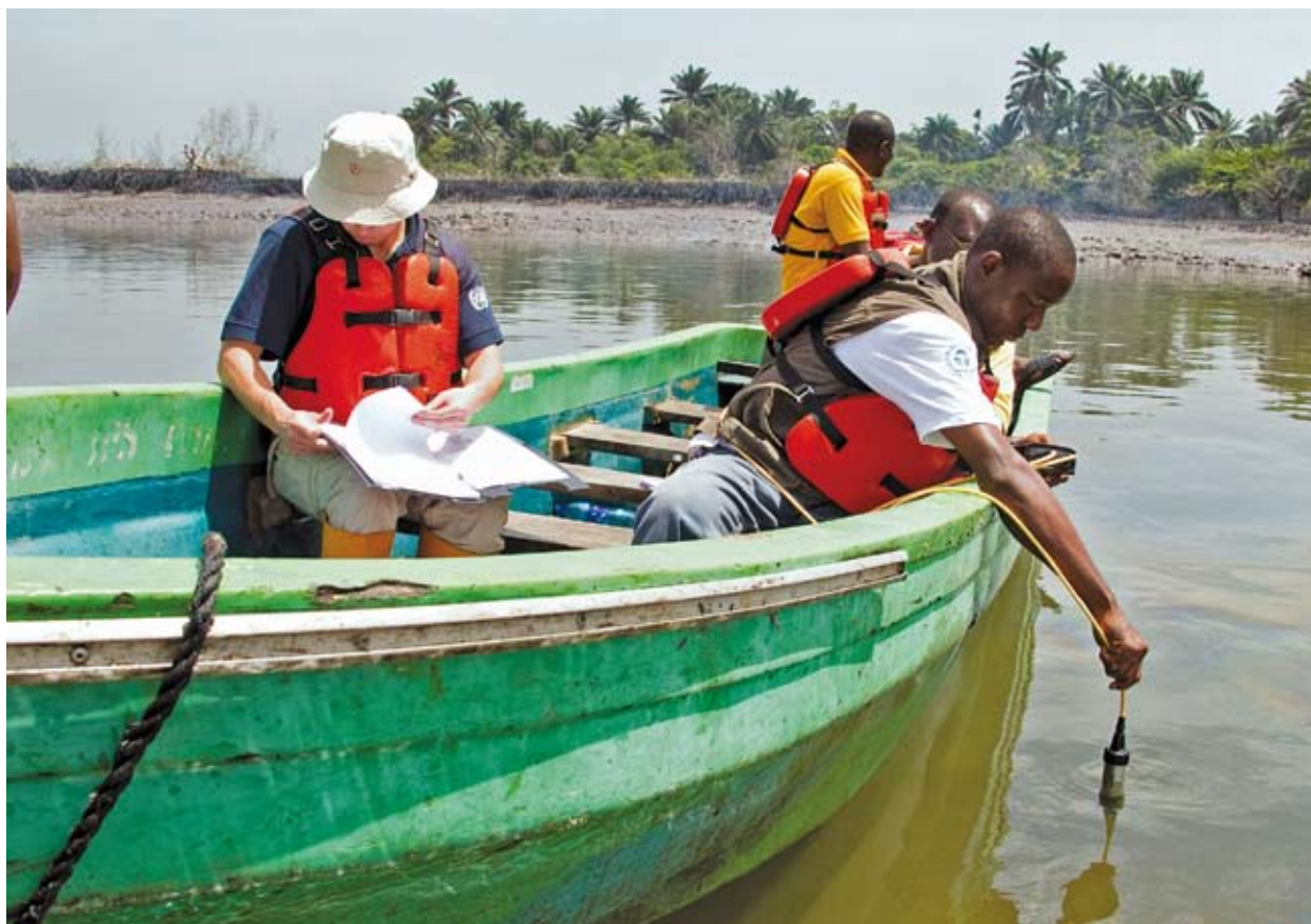
During and following clean-up operations in Ogoniland, a monitoring programme should be put in place which includes monthly monitoring of surface water and quarterly monitoring of sediments
