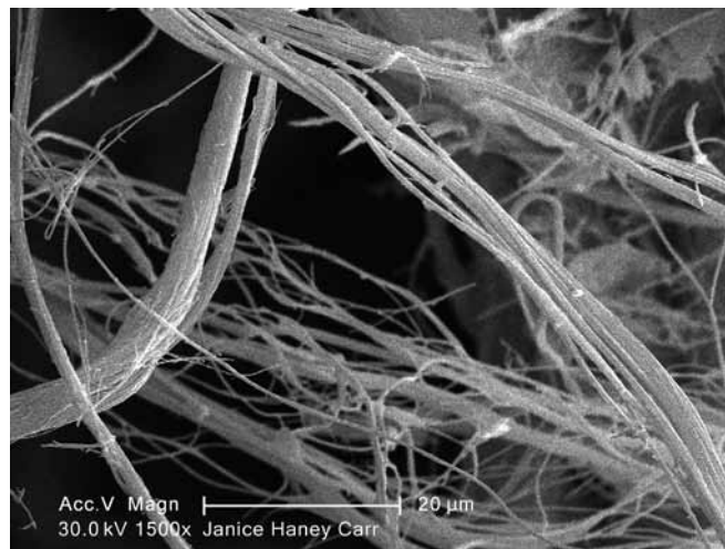
Asbestos fibres magnified 1500 times under scanning electron microscope
