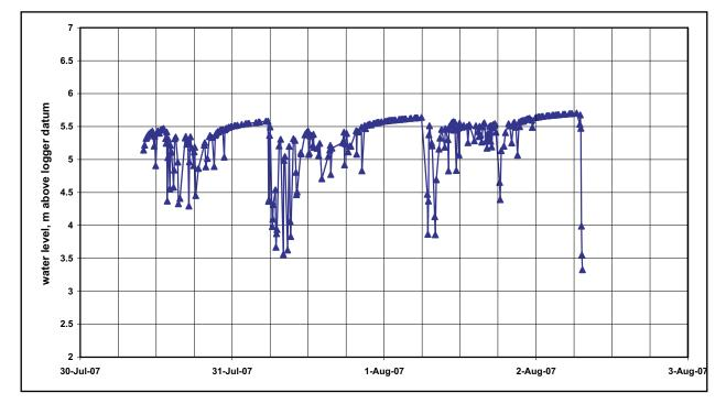
over four days in July-August 2007. There are similarities with the records from other pumped wells, but in this instance the rate of pumping is much lower and the individual pumping episodes much shorter. This has resulted in a very 'spiky' pattern. It is clear that the water level recovers fully overnight, and even over the short period shown, it can be seen that there is a small rise in the rest water level, of about 0.1 m.
