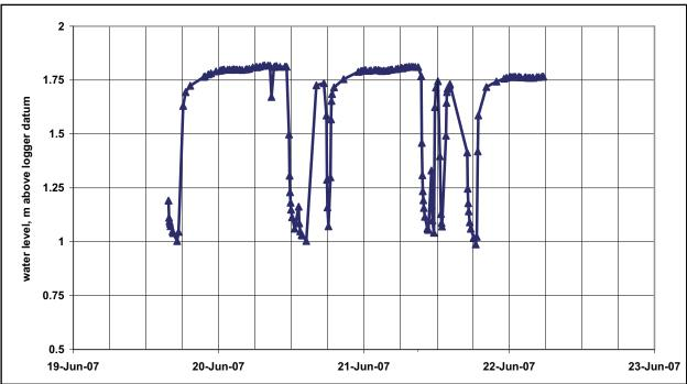
Figure 14. Oxfam Logger, Al Shahied Dug Well, Kebkabia, North Darfur – Four days
