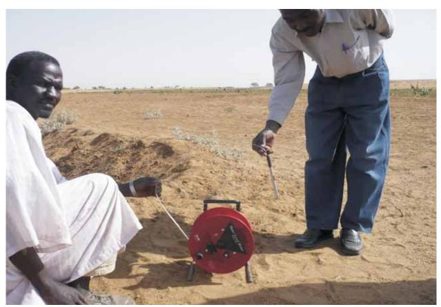
Figure 8. A "dipper" for manual measurement of water in a well. The sensor is on the end of a tape dropped down the well for a manual reading to water depth.
